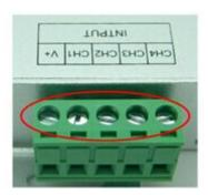
V+: 12V/24V: signal input common anode common public pole CH1/CH2/CH3/CH4: signal input cathode R/G/B/W channel
