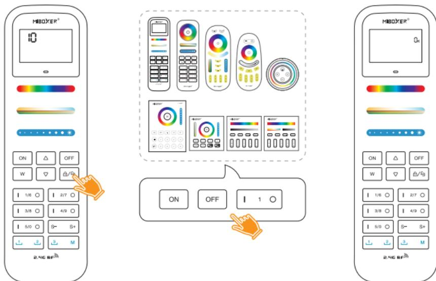
1. Short press “ON” 5 times quickly to enter into copying mode, LCD screen display “countdown 10 seconds”
